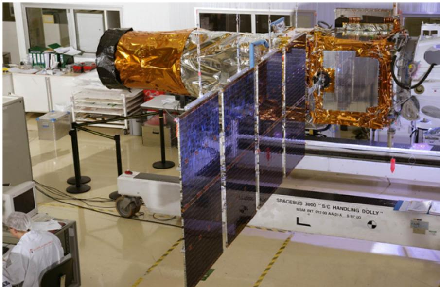
**Fig. I.3.4.** The CoRoT telescope, during the final tests (opening of the solar panels) at Alcatel (Cannes), © Thales Alenia Space.
