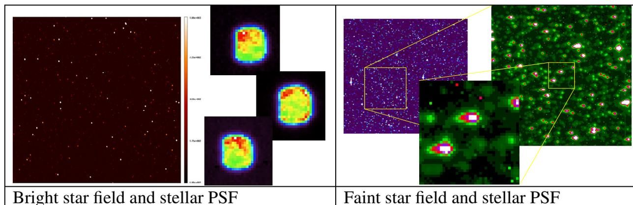
**Fig. I.3.5.** Point spread functions in the two CoRoT fields, with the very broad stellar images in the bright star field (to improve the accuracy of the photometry) and the smaller faint star images in the faint star field, enlarged by the very low resolution prism to extract color information, © CNES.
