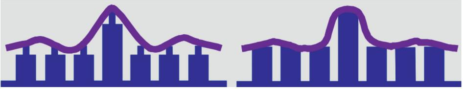
**Fig. 8.** Deformable mirror fitting illustration. (From Riccardi 2003.)
