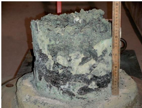
Figure 5.49. Appearance of the resolidified lump of corium at the end of the SSWICS-11 test, performed with gas injection into the corium, see [32]; reproduced by permission of OECD.
