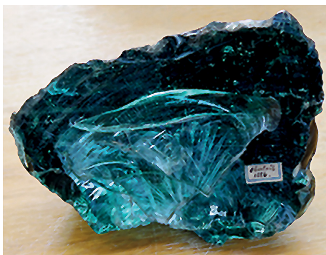
Figure 2.7: Chunk of glass discovered close to the Roman settlement Nauportus, presently Vrhnika in Slovenia [40]. Analysis based on the PIXE-PIGE method demonstrated that the material was natron-type glass characterised by sub-percent concentrations of \text{MgO} and \text{K}_2\text{O} . This indicates that the material represents primary Roman raw glass intended for further reworking in secondary workshops.
