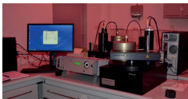
Figure 4.1: Equipment used to measure TL (thermo-luminescence) and OSL (optically stimulated luminescence) in a dating laboratory.
