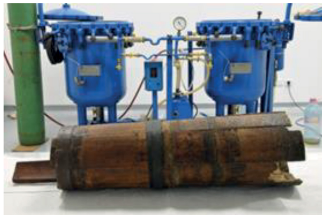
Figure 6.8: Test consolidation facility at IRASM IFIN-HH: 100 liter vacuum/pressure impregnation equipment (back); wooden butter churn degraded by woodworm attack and consolidated by radio-polymerisation (front).
