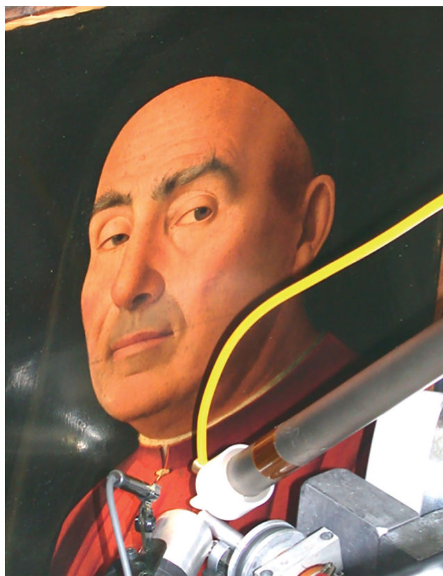
Figure 2.17: The painting Ritratto Trivulzio by Antonello da Messina (15 th c.) during measurements at the LABEC external microbeam in Florence.
