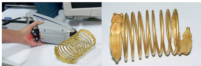
Figure 2.12: Dacian spiral gold armbands studied by XRF analytical methods.
