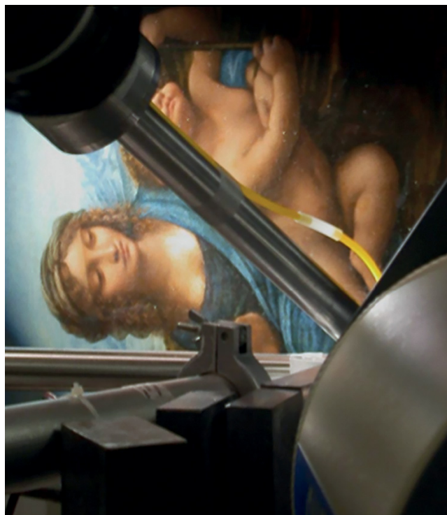
Figure 2.15: The Madonna dei fusi at the PIXE-PIGE set-up in Florence.
