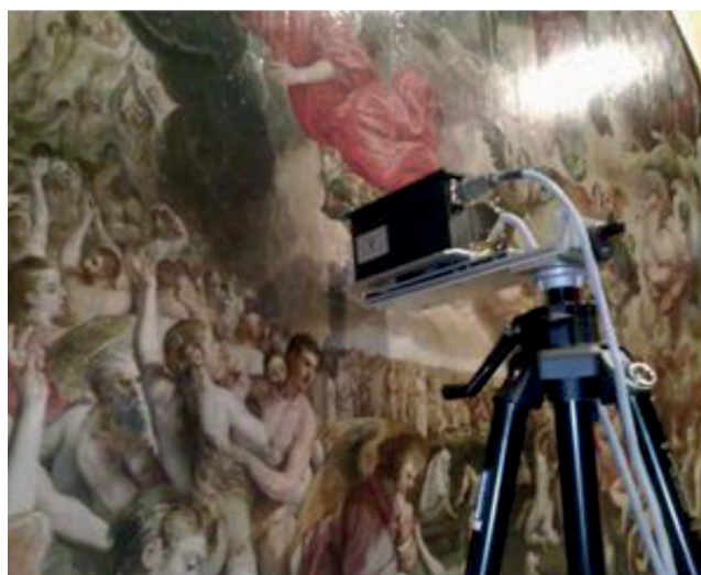
Figure 5.6: Analysis of pigments in situ by a portable XRF device.
