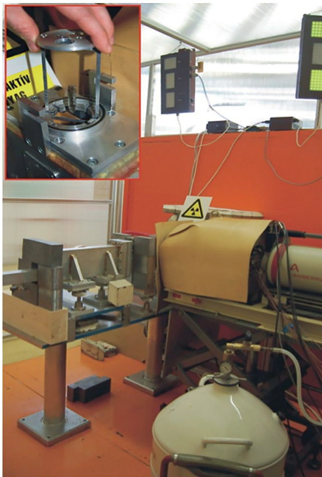
Figure 3.1: The Prompt Gamma Activation Analysis facility at the Budapest Neutron Centre. Insert photograph: A sample holder with a small obsidian sample.
