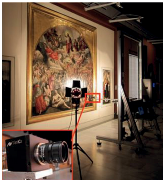
Figure 5.5: The triptych analysed in situ by IRR, placed on a semi-automatic support. The inserted image shows the InGaAs camera.
