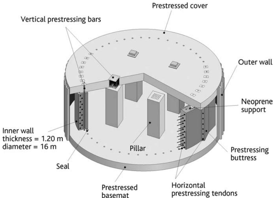
Figure 10.19 Diagram of the MAEVA mock-up. © Georges Nahas/IRSN.
