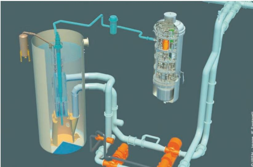
Figure 2.1 Diagram of the CABRI safety test reactor with its pressurized water loop.
