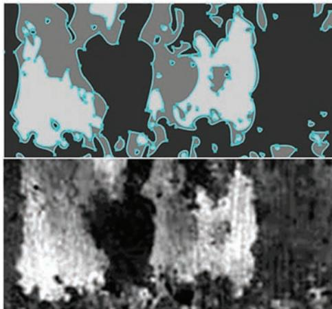
**Figure 10.14** Example of grain-shape recognition for cast steel fabricated by Manoir. © IRSN.
