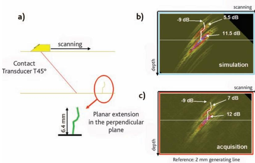
**Figure 10.11** Ultrasonic response of a multifaceted defect during contact examination using 45° transverse waves. a) examination configuration; b) "simulated" defect image; c) "experimental" defect image. © DR.
