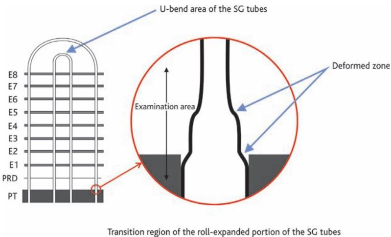
**Figure 10.6** Another example of complex geometry: the transition region of the roll-expanded portion of the steam generator tubes and the <sup>191</sup>U-bend areas of the tubes. © IRSN.
