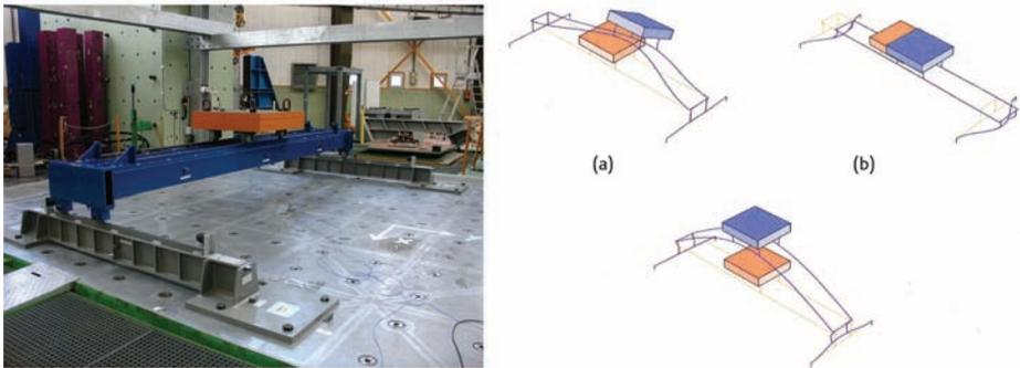
**Figure 10.15** Overhead crane tested on the AZALEE table (left) and the three main modes of deformation obtained by numerical simulation. © CEA (left).
