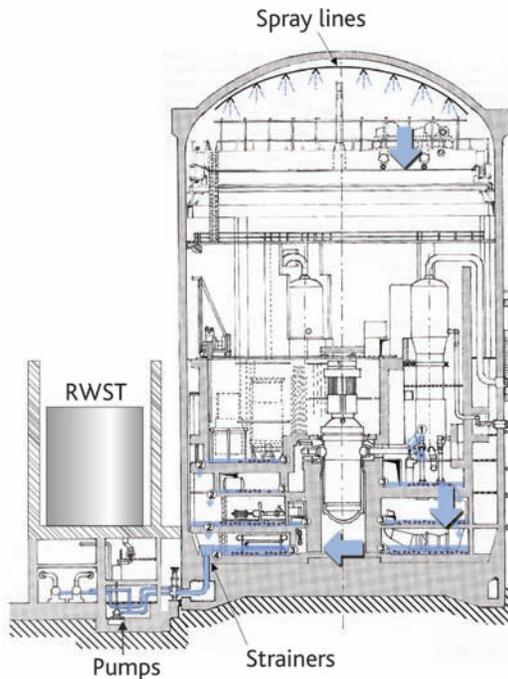
**Figure 5.2** Illustration of debris transport to sump strainers (900 MWe PWR containment building).
