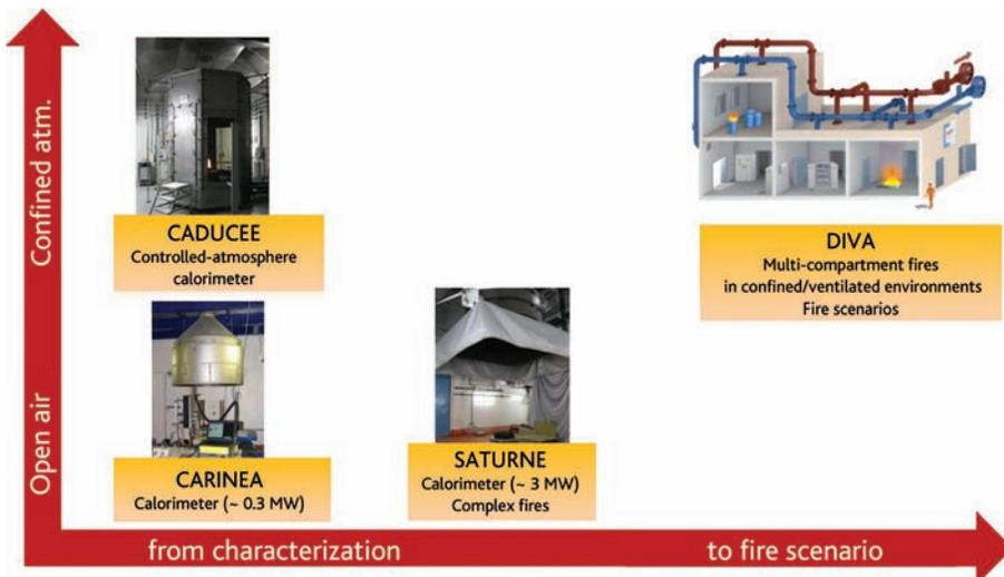
Figure 7.2-a Positioning of the different types of fire characterization test in relation to the test facilities.
