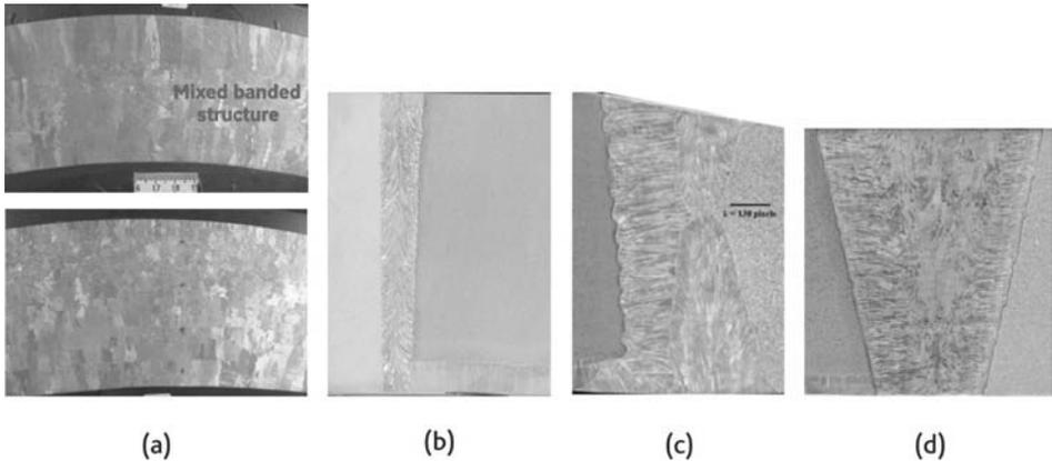
**Figure 10.13** Coarse-grained metallurgical structures observed on IRSN mock-ups representative of: (a) a cast component fabricated by Manoir; (b) a narrow groove weld; (c) stainless steel bimetal bond fabricated by Cockerill; (d) "N4" vessel bimetal bond. © IRSN.
