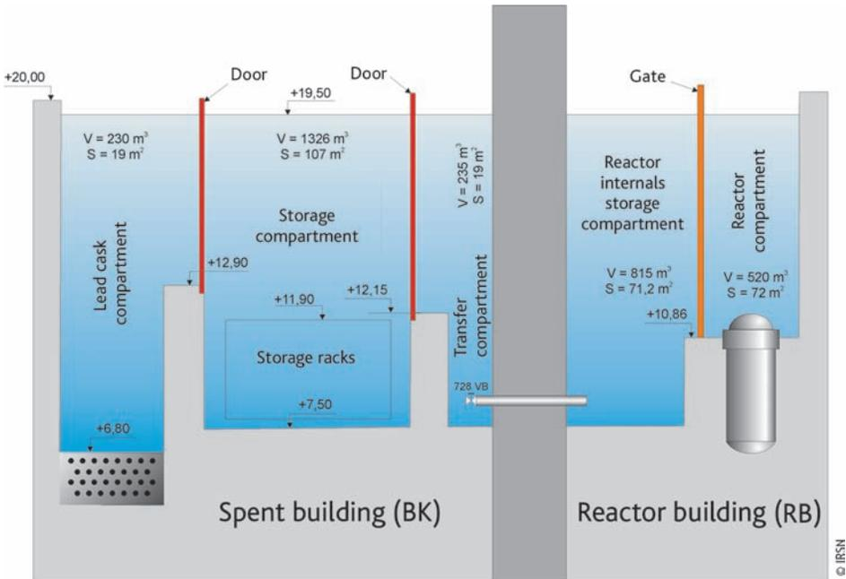
**Figure 6.1** Cutaway view of the reactor cavity in the reactor building (RB) and the spent fuel pool in the fuel building (BK) in a 900 MWe CPY<sup>48</sup>-series plant.
