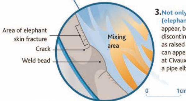
3. Not only can surface cracks (elephant skin fractures) appear, but isolated cracks, located at discontinuities deeper in the metal, such as raised surfaces formed by weld beads, can appear. In 1450 MW reactors like the one at Civaux, the problem was compounded by a pipe elbow and welds in this zone.
