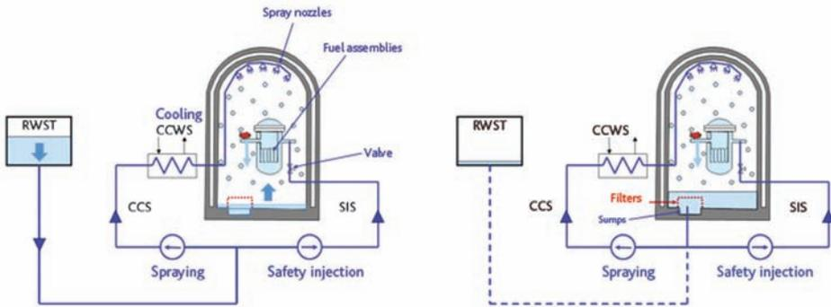
**Figure 5.1** Simplified diagram of SIS and CSS operation in direct injection mode (left) and recirculation mode (right) – the component cooling water system (CCWS) is also responsible for cooling some pumps in the systems shown. © IRSN.
