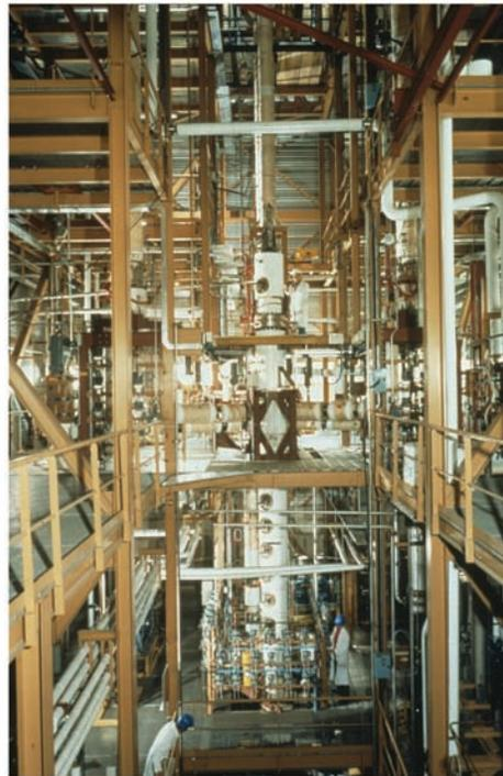
Figure 3.1 The BETHSY loop (900 MWe PWR, three loops). © Georges Goué/IRSN-Source CEA (left), CEA (right).
