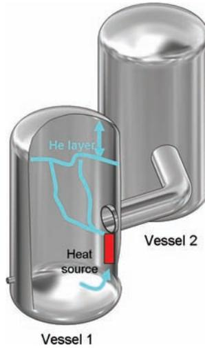
Figure 9.6a Diagram of the PANDA facility. © PSI.
