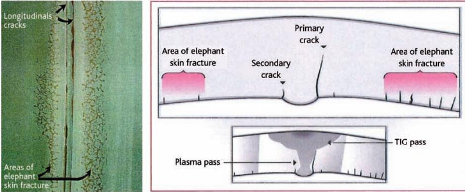
**Figure 10.2** The inside of the pipe elbow that caused the leak that occurred at the Civaux NPP in 1998. Crazing-like fractures are visible on either side of the weld bead. © EDF (left) and IRSN—Source: EDF (right).
