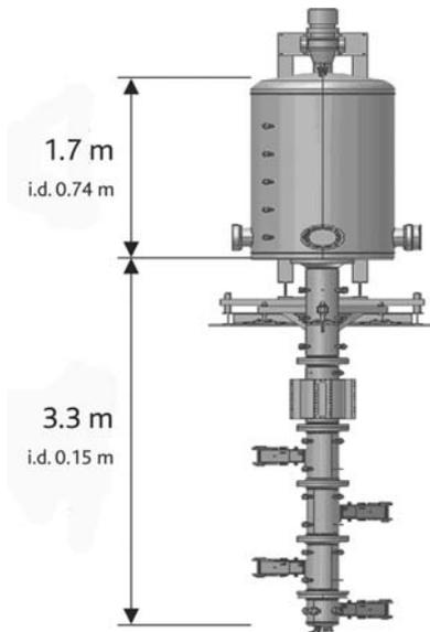
Figure 9.8 Diagram of the ENACCEF facility [16].
