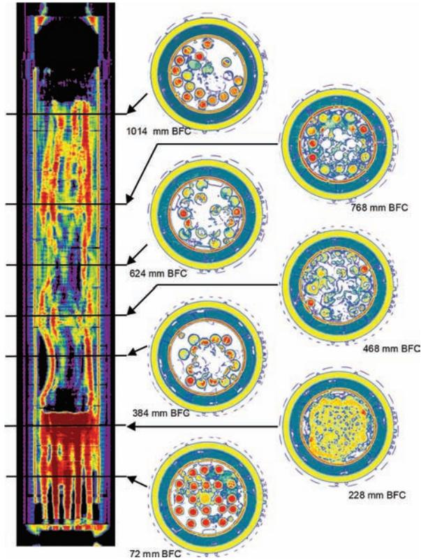
**Figure 9.3** State of degradation of a fuel assembly after test FPT1; post-test non-destructive examinations of the tested fuel cluster: X-ray (left) and X-ray transmission tomography (right). (BFC: Bottom of Fissile Column). © IRSN.
