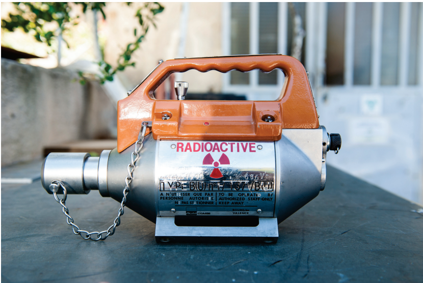
Figure 25. Gamma radiography projector containing a radioactive source, France. © Nedim Imré/IRSN.
