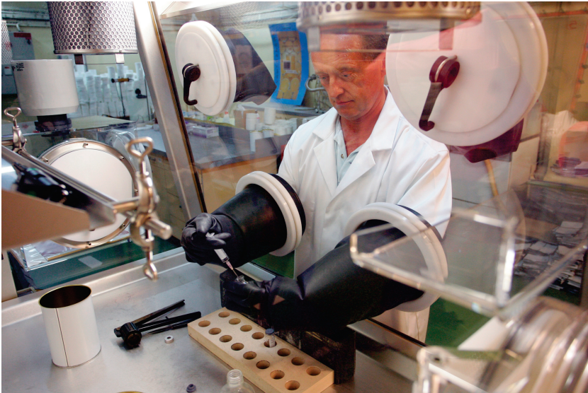
Figure 23. Reconditioning radioactive sources at IRSN, Fontenay-aux-Roses, France. © Olivier Seignette/Mikaël Lafontan/IRSN.
