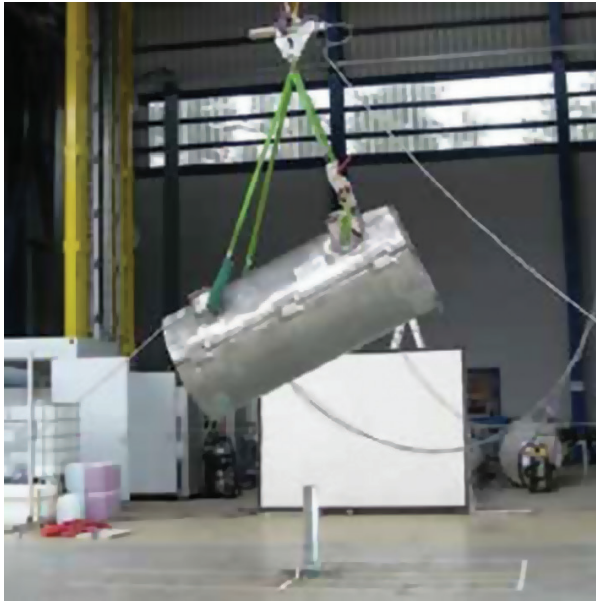
Figure 11.2. Drop test on a (vertical) punch bar of a Daher-NCS DN30 package model (type B package). ASN.
