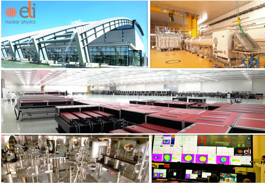
FIG. 7.4 – Upper row, left: ELI-NP special building, that hosts the laser system and the experimental areas. Upper row, right: E1 experimental chamber for 2 \times 10 PW pulses and the beam transport for the long focal distance mirror for 10 PW pulses at E6 experimental area. Middle row: laser room, hosting the two laser amplification arms; Lower row, left: inside the 1 PW experimental chamber in E5 experimental area; lower row, right: the large screen in laser control room showing synthetic information on the HPLS status.
