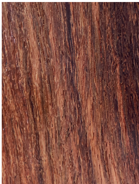
Pterocarpus erinaceus Longitudinal surface of wood
