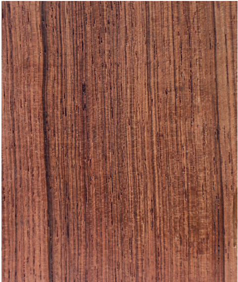
Dalbergia stevensonii Longitudinal surface of wood
