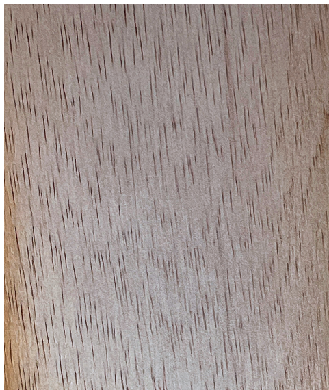
Falcataria moluccana Longitudinal surface of wood
