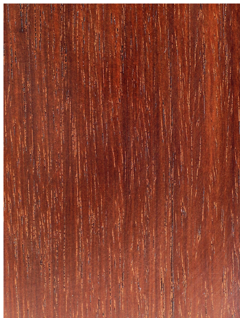
Pterocarpus santalinus Longitudinal surface of wood
