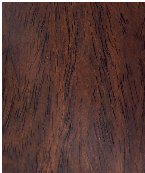
Dalbergia retusa Longitudinal surface of wood
