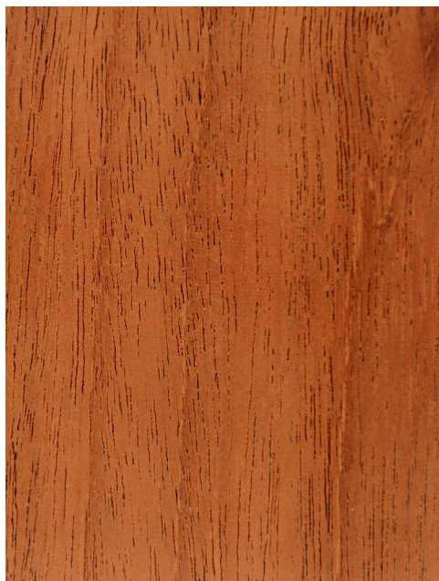
Swietenia macrophylla Longitudinal surface of wood
