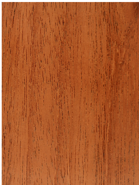
Swietenia mahagoni Longitudinal surface of wood
