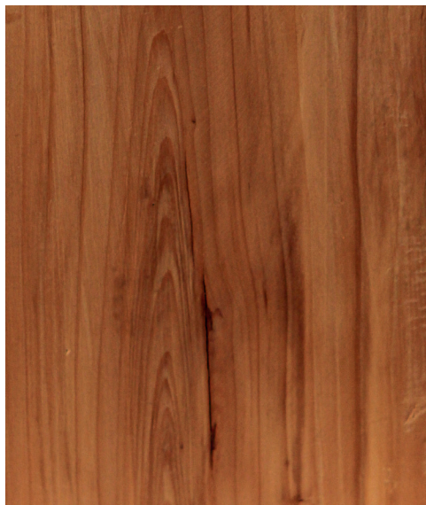
Pseudotaxus chienii Longitudinal surface of wood
