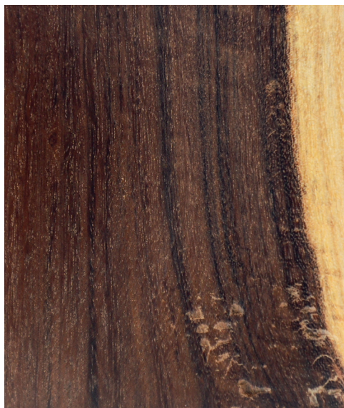
Guibourtia conjugata Longitudinal surface of wood
