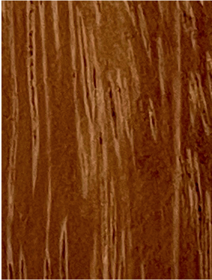
Anadenanthera macrocarpa Longitudinal surface of wood
