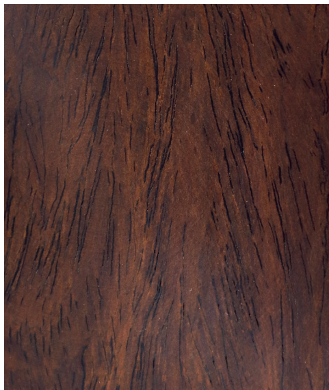
Dalbergia retusa Longitudinal surface of wood
