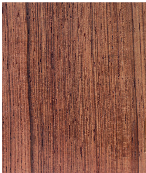
Dalbergia stevensonii Longitudinal surface of wood
