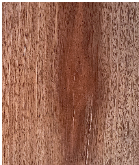
Khaya senegalensis Longitudinal surface of wood
