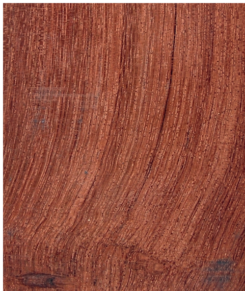
Guibourtia pellegriniana Longitudinal surface of wood
