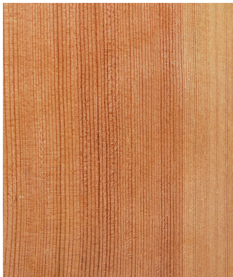
Pinus sylvestris var. mongolica Longitudinal surface of wood
