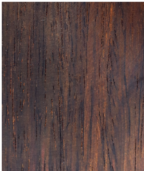
Dalbergia granadillo Longitudinal surface of wood
