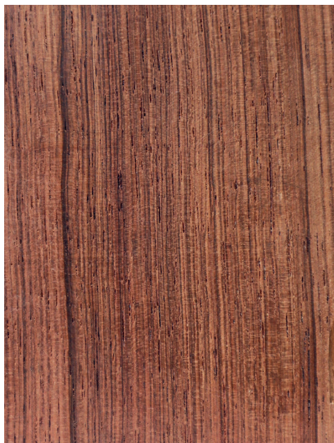
Dalbergia stevensonii Longitudinal surface of wood
