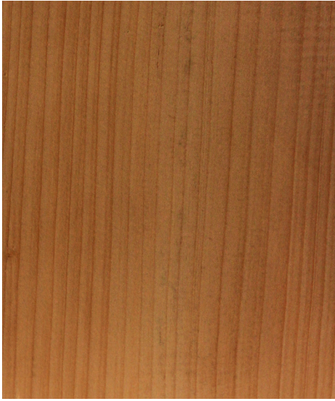
Torreya grandis Longitudinal surface of wood
