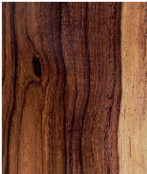
Dalbergia tucurensis Longitudinal surface of wood
