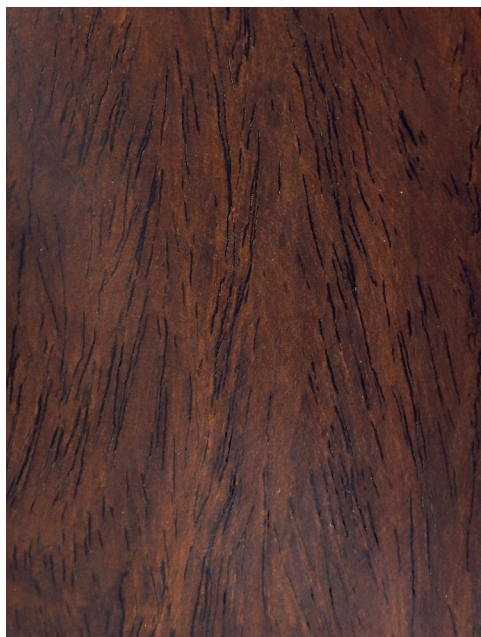
Dalbergia retusa Longitudinal surface of wood
