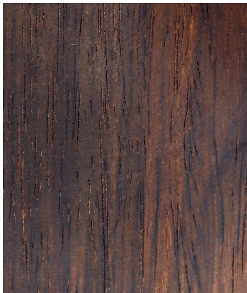
Dalbergia granadillo Longitudinal surface of wood
