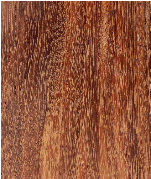
Dalbergia sissoo Longitudinal surface of wood
