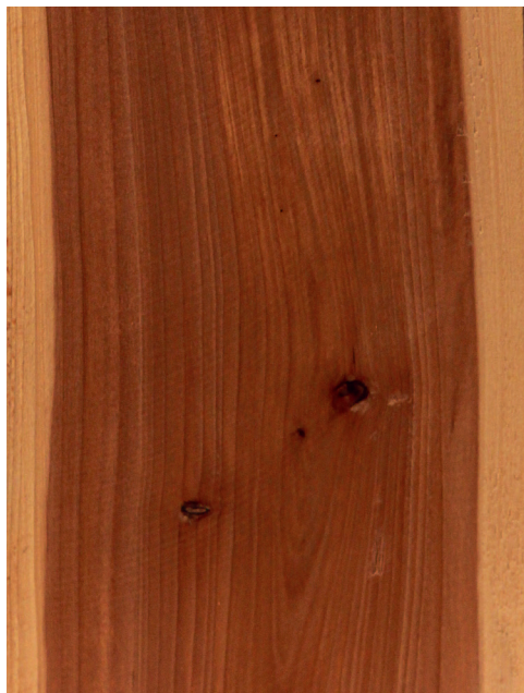
Taxus chinensis Longitudinal surface of wood
