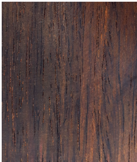
Dalbergia granadillo Longitudinal surface of wood
