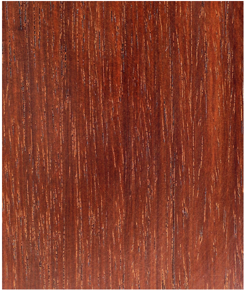
Pterocarpus santalinus Longitudinal surface of wood
