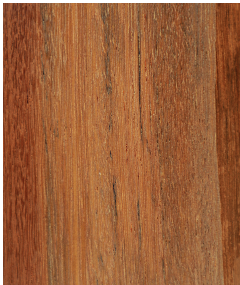
Guarea grandifolia Longitudinal surface of wood
