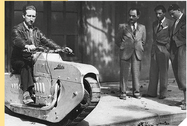
Prototype "Lehaître" for a tracked caterpillar motorcycle (1938)
