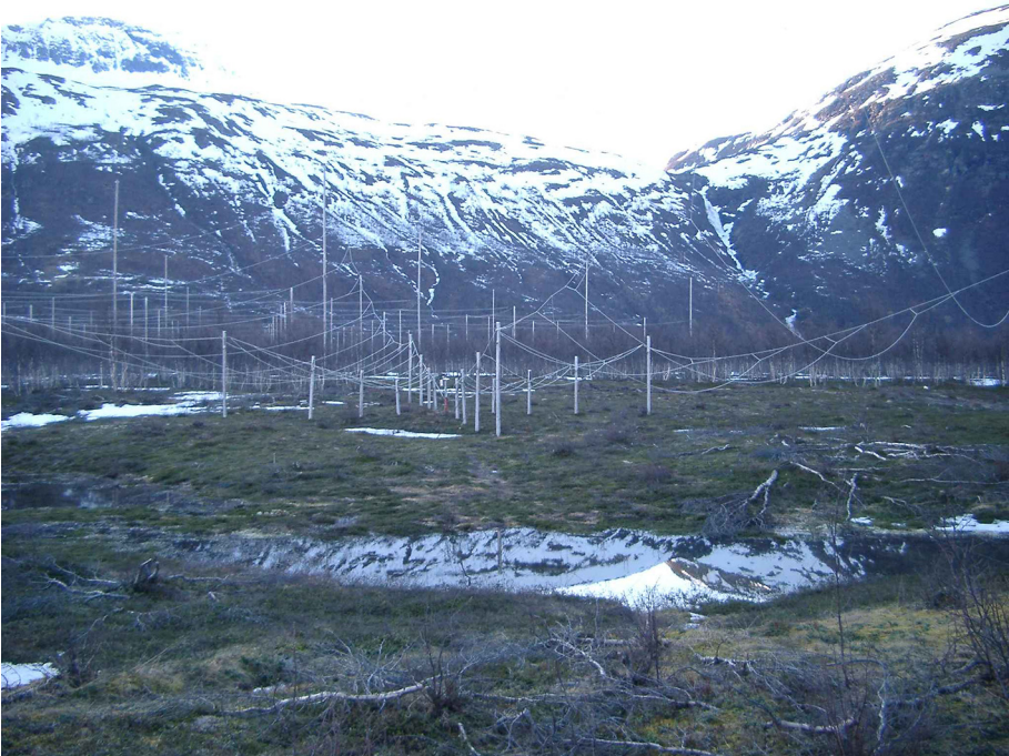
FIG. 3.12 – A dynasonde in Norway, near the Ramsfjörd (credit: M. T. Rietveld, EISCAT Scientific Association).
