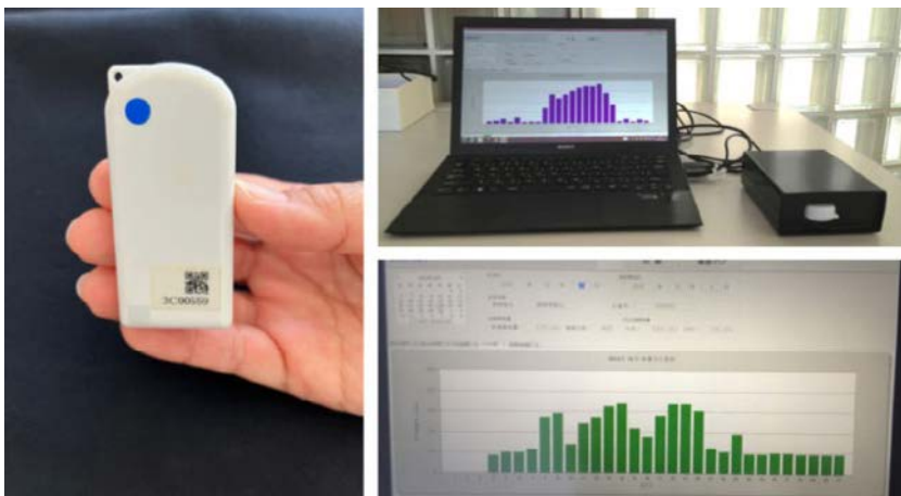
FIGURE 2. The left side shows the D-shuttle device. The upper right shows the management unit and an example of hourly dose display, while the lower right shows the daily dose (photos: W. Naito).
